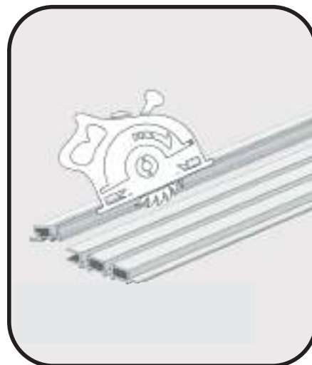
04. Cut the wall Panels to fit the remaining length.
