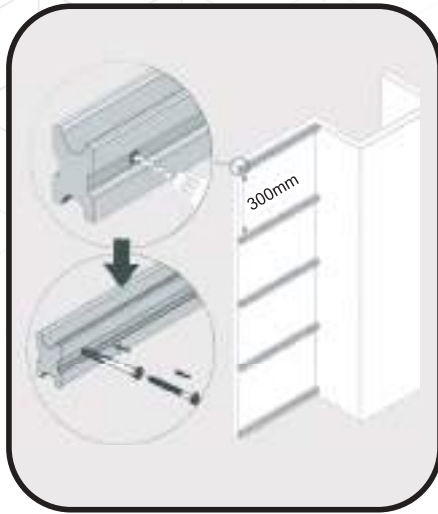
01. Install the framing profile / Aluminum channel horizontally using expansion screws, with a spacing of 300 mm between the framing profile / Aluminum strip
