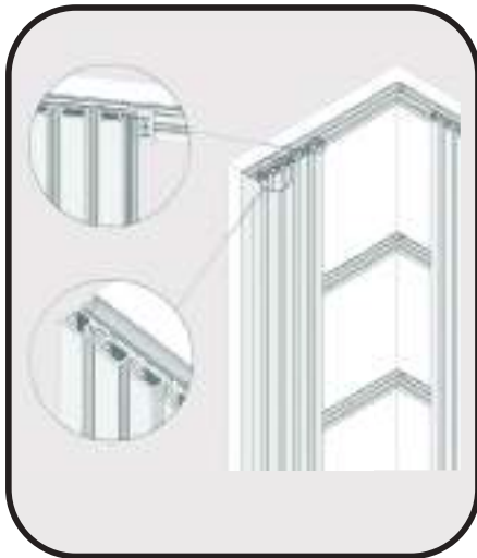
03. Install the wall panels sequentially from both sides, securing them with metal clips.
