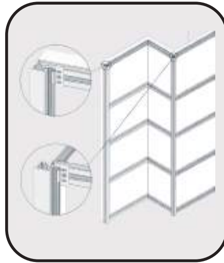
02. Use metal clips to install and secure the exterior corner and corner profile.
